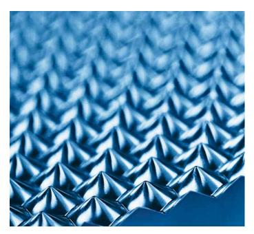
CDPS is an enhanced conical prism structure that offers even more effective de-glaring in the plane of the sheet when compared to the standard CDP structure. The CDPS is used specifically in combination with a plane transparent sheet underneath the structured side, thus offering an even stronger de-glaring as well as a smooth outside surface and therefore less sensitivity towards dirt and staining with easy cleaning. This is especially beneficial for medical or other hygienic applications.
